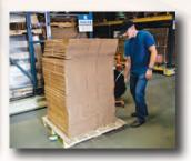
Strap threading with the SFT is fast, accurate and significantly reduces stooping and kneeling.
